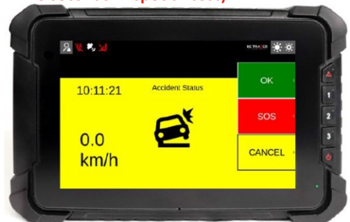
Probable accident screen (appears after a stop of at least 15 seconds in special test)
